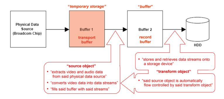
TiVo's diagram omits *four* claimed elements that *must* occur between the *temporary storage* and the *buffer*—namely, *extraction*, *conversion*, *fill*, and *automatic flow control*.
